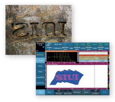
Scanning on pipe (wall thickness 4mm)
