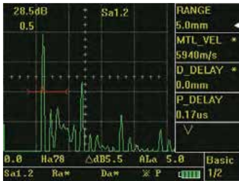
(Bottom echo of a 1.2mm steel plate)
